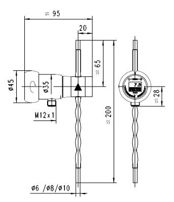
A spacer between the electronics head and the medium-contact measurement tube provides thermal decoupling between the two units. The media temperature may be raised for 45 min. to 130 °C.
