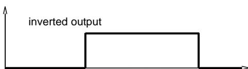
A Power-On delay function (ordered as a separate option) makes it possible to maintain the switching output in the normal state for a defined period after application of the supply voltage.
