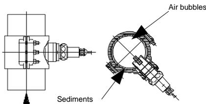
The best installation position (low contamination, good venting) is with the direction of flow from bottom to top, or in horizontal piping with the sensor at an angle of  $45^\circ$  downwards. The union nut must be tightened to a torque of 30 Nm.
