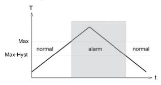
A switchover delay time ( $t_{DS}$ ) can be applied to the switchover to the alarm state. Equally, one switch-back delay time ( $t_{DR}$ ) of several can
