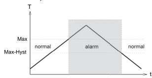
The change to the alarm state is indicated by the integrated red LED and a cleartext in the display.
