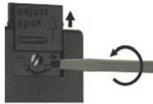
Turn clockwise for a lower switching point; turn anticlockwise for a higher switching point. After adjustment, close the slider again.
