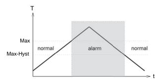
A switchover delay time ( $t_{\text{DS}}$ ) can be applied to the switchover to the alarm state. Equally, one switch-back delay time ( $t_{\text{DR}}$ ) of several can be applied to switching back to the normal state.
